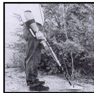
Once you have got a steady threshold, quickly lower the coil straight down to approximately 1 inch off of the ground.
