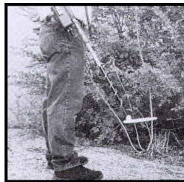
Lift your detector straight off of the ground about 6 to 8 inches. Keep the coil parallel to the ground.
