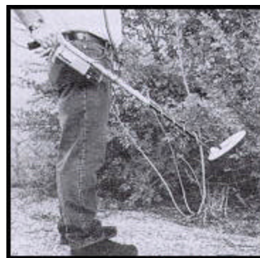
You must lift your coil straight up. Do not swing it like a pendulum.
