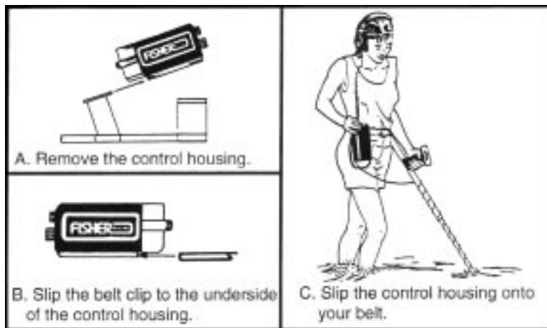
Figure 6. You can hipmount your CZ-20 by sliding the control housing from the handle and attaching it to your belt. This reduces the weight of the stem, creating nearly effortless hunting.
